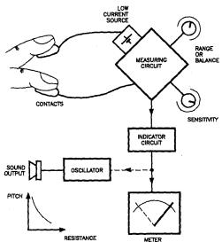
Figure 3. General arrangement of a Galvanic Skin Resistance meter, or GSR. Both meter and sound output may be used. A very low current is passed through the skin (you can't feel it) — usually between two fingers or in the wrist area. The range or balance control is set to bring the reading on-scale because actual skin resistance differs widely from person to person and time to time. Sensitivity is adjusted to show the required response.
