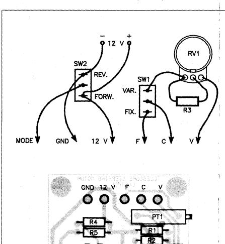
The assembly can proceed in any order. However, the two links should be soldered in place first; one of them is beneath the 555. Make sure you place the ICs facing the right direction – in each case, pin 1 faces toward the trimpot. Capacitors C2 and C3 are polarised, so make sure you solder them in the right way round, too.
