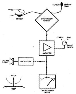
Figure 4. Diagram showing how a skin temperature biofeedback instrument works. Two sensors are used, one measuring ambient temperature, the other measuring the temperature of the skin in the area where it is located. The two sensors' outputs are compared, the differences amplified and applied to a centre-zero meter. Sound output feedback may also be provided.
