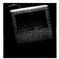
Skin Temperature biofeedback meter, by Thought Technology. This model has analogue meter readout.
