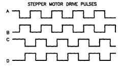
Figure 2. Showing the operating pulses required by unipolar stepping motors. The A-B-C-D pulse sequence is output from pins 6, 8, 9 and 11, respectively, of the SAA1027 in the controller circuit.
