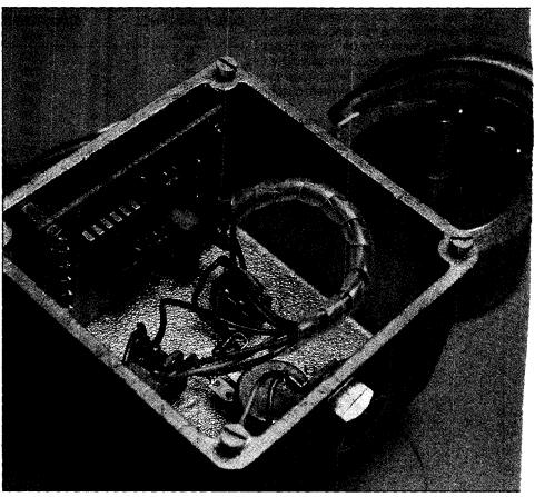
Showing the completed board mounted in a diecast box, and the stepping motor it controls.
