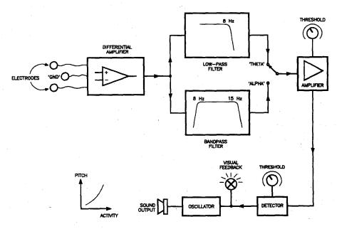
of low amplitude, measuring a few microvolts, the signals can be quite easily sensed using electrodes on the skin and filters to select the desired brain wave pattern. Figure 6 shows a typical brain wave blofeedback instrument.
