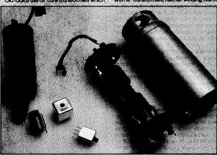
RF coils and transformers. At left a 1930s valve radio (wireless) coil contrasts with a modern RF coil in front of it. In the centre are two modern RF transformers, while an earlier valve radio IF transformer is shown at right outside its shield can.
