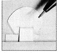
Showing the tongue that activates the switch on the melody module hidden inside the card.
