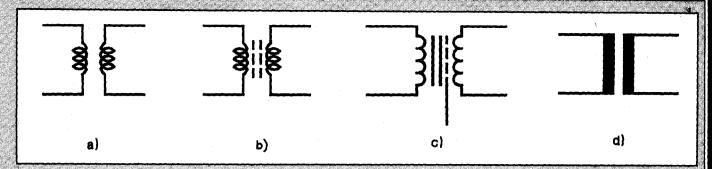
Figure 3.1 Symbols for transformers. s) untuned RF or IF transformer; a tuned version would have a capacitor connected across the secondary and/or primary; b) ferrite-cored transformer, RF, IF, or sometimes audio; c) Iron-cored transformer, audio or power frequencies. The deshed line represents an electrostatic shield; d) power transformer.
