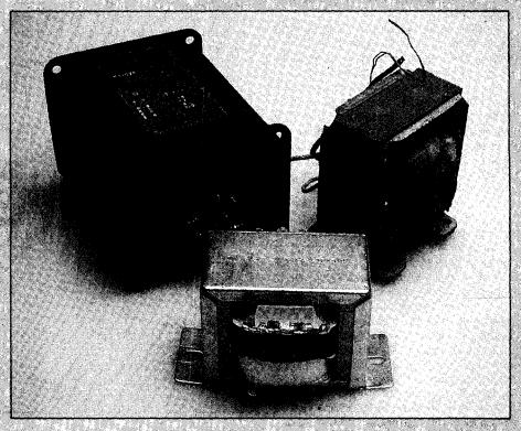
A trio of transformers! At left rear is an audio output transformer (once Australian made). At right is an ancient power transformer, in front is a common multi-tap low voltage transformer.
