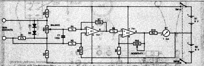
Circuit diagram of the ETI-1545 GSR Meter. Despite the obvious simplicity, it's a sensitive and functional instrument.
